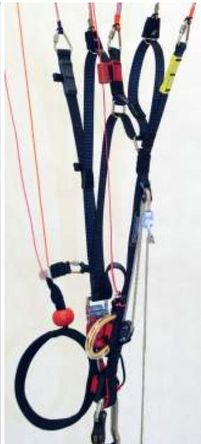
The pulley in 3rd position with closed trimmer; EK magnet is fixed above the carabiner
