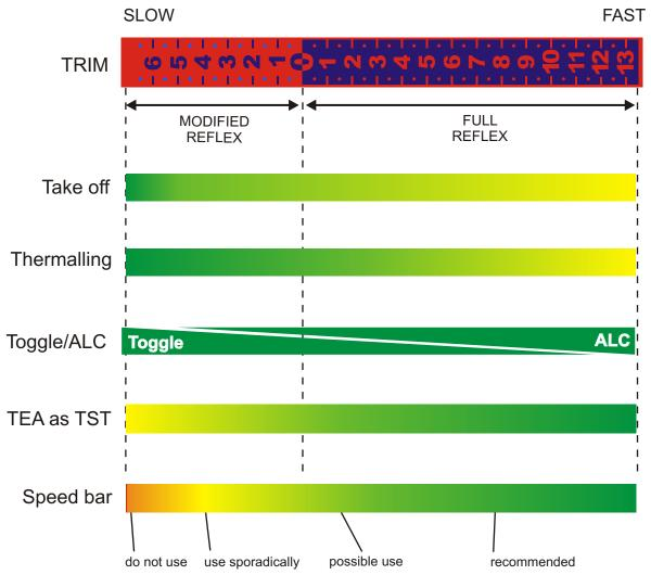
In null-wind conditions the easiest way to take off is to keep trims closed. The stronger the wind, the more should they be advanced towards '0' position. At faster trim settings take off can be hard to impossible (depending on wind strength).
